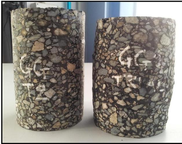
**Figure 2** – AMPT specimens after FN testing
